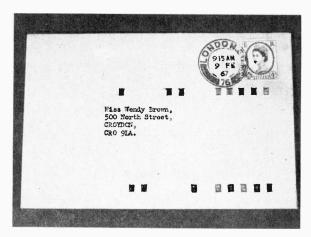
Fig. 1. A typical postcode pattern. The dots imprinted at the coding desk are normally almost invisible to the naked eye and have been outlined here
