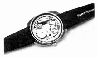
the mechanical vibrator 170 times per second. This correction is carried out by a relatively simple circuit employing only 14 transistors, 19 resistors and seven capacitors. The logical deductions made by this circuit are fed to the motor as correction signals. This watch is said to be the first cybernetic watch, since it employs a comparison circuit or "brain".
