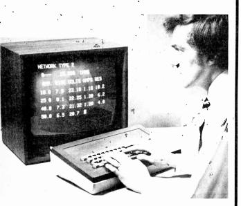
This display system developed at the Mullard Central Applications Laboratory can display up to 16 rows of 80 characters, each character being generated on a 7  $\times$  5 dot matrix
