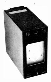
A digital indicator using the Perspex light-guide technique as described in Fig. 3.2 (supplied by Electronic Brokers Ltd.)
