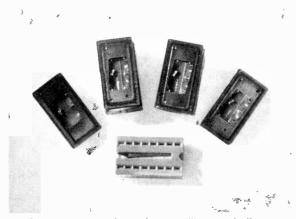
Seven segment incandescent filament indicators in dual-in-line packages (Minitron 3015F, available from A. Marshall & Son)
