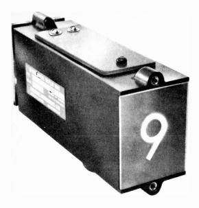
A rear projection type display unit. This type gives 1in characters using 6:3V pilot lamps. It will give all the numerals and a decimal point (supplied by Electronic Brokers Ltd.)
