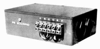
The completed electronic ignition unit in a diecast box. Note the terminal block and power transistors with plastics covers
