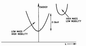
Fig. 12. Energy band diagram for gallium arsenide
