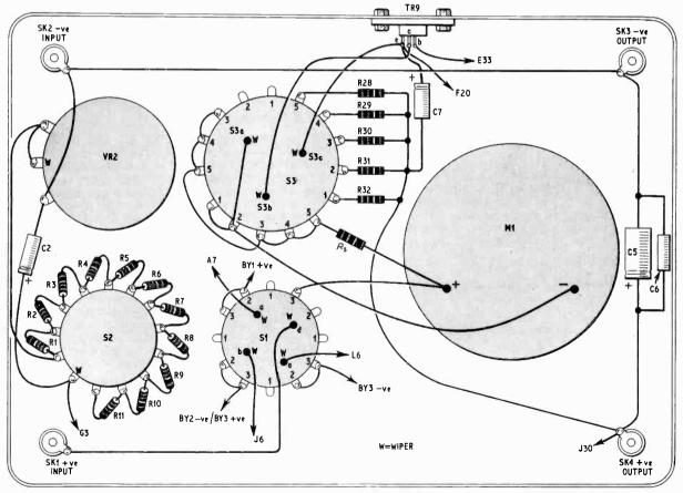
Fig. 5. Internal wiring of the stabiliser
