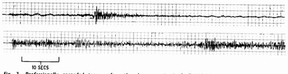
Fig. 3. Professionally recorded traces of earthquakes occurring in the British Isles. Upper trace: earthquake at Glen Spean in Scotland; lower trace: earthquake under South Downs in England (Photo by courtesy U.K.A.E.A. Blacknest)
