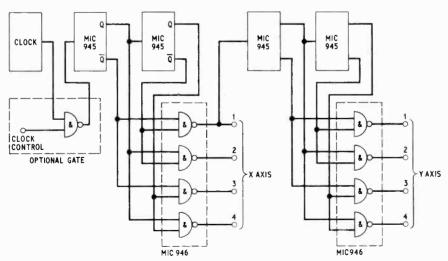
Fig. 3. Using the output from one of the gates of Fig. 2 to drive an identical system, we can sequentially switch on every lamp in turn in a 4 imes 4 lamp matrix
