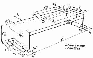
Fig. 5. Panel bridge for mounting the various stage panels
