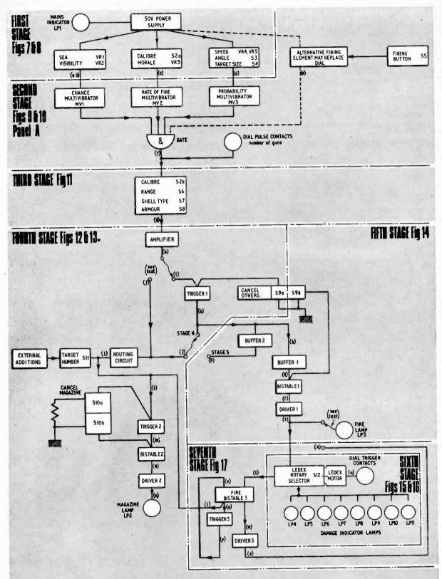
Fig. 3. Block diagram of the complete war game computer with alternative operational modes for smaller systems. The equipment is built up in stages, each stage being a workable progression from the previous
