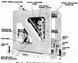
Fig. 4. A professional seismometer
