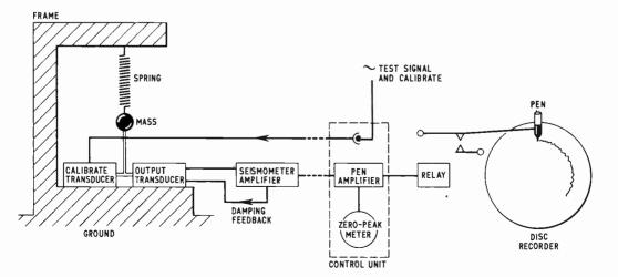
Fig. 1. Block diagram of seismograph
