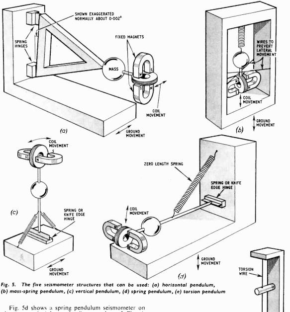
the same principle as the Sprengnether of Fig. 4. Resonance is adjusted by sliding the mass along the boom, and moving the spring anchoring points. A special spring must be employed for best results, and the boom pivots on a strip hinge or knife edge.
