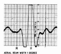
Fig. 3.5. Recording of the sun obtained from the aerial system shown in Fig. 3.4 used in conjunction with a phase-switched receiver
