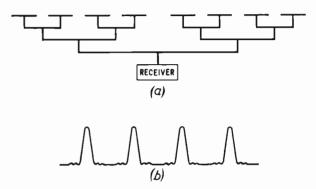
Fig. 3.4. A grating interferometer: (a) arrangement of aerials; (b) reception pattern
