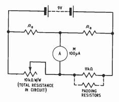
Fig. 3. Wheatstone bridge for resistor matching
