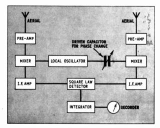
Fig. 3.3. Rotating lobe interferometer
