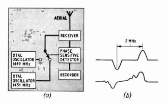
Fig. 3.9. The detection of spectral lines: (a) the switched comparison receiver; (b) typical outputs from receiver
