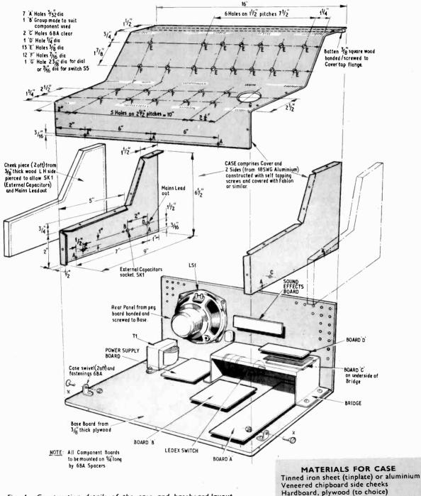
Fig. 4. Construction details of the case and baseboard layout
