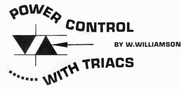
TRIAC is the name used to identify the triode a.c. semiconductor bidirectional switch. It is basically two reverse blocking triode thyristors or silicon controlled rectifiers connected in inverse parallel, but with a common control electrode (gate). As the triac is a development of the thyristor, it is logical to describe this first and then compare with the triac to show the advantages and disadvantages of both devices.
