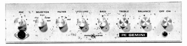
Photograph of the front panel showing control designations
