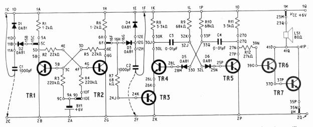
Fig. 6.1. Gated alarm circuit with  $\mu$ -DeC connections. The bistable TRI and TR2 triggers a relaxation oscillator TR4 and TRS via TR3. The sound is amplified by TR6 and TR7 and fed to an 80 ohm loudspeaker. Positive and negative trigger pulses are supplied by the connection of CI or C2 to either supply rail
