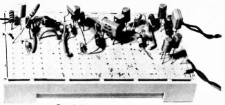
Gated alarm circuit made up on  $\mu$ -Dec
