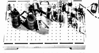
Square wave generator and -2 divider made up on T-Dec
