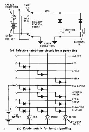
Fig. 2.7. Two examples of other uses of the diode
