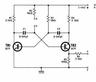
Fig. 1. Circuit of tone generator
