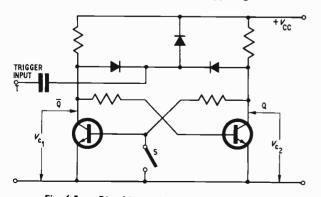
Fig. 6.3a. Bistable used as a binary divider
