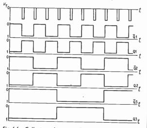
Fig. 6.6. Collector voltage waveforms of the binary counter
