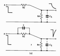
Fig. 6.2b. The effect of applying commutating capacitors to overcome the stray capacitors  $C_s$
