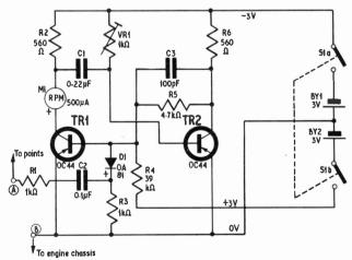
Fig. I. Circuit diagram of the marine tachometer
