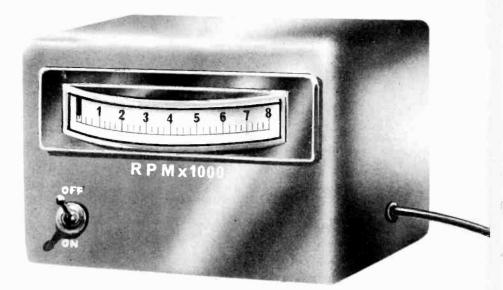
Completed tachometer housed in a water resistant case, showing the linear meter scale for a maximum r.p.m. reading of 8,000
