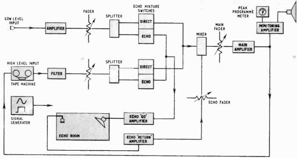
Fig. 1. Typical block diagram of a sound effects set-up for adding effects to a programme
