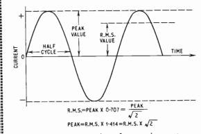
(a) Peak and r.m.s. values of an a.c. sine wave. 11 cycles are shown
