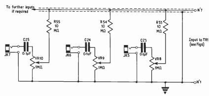
Fig. 19. Extension circuit for more than two inputs
