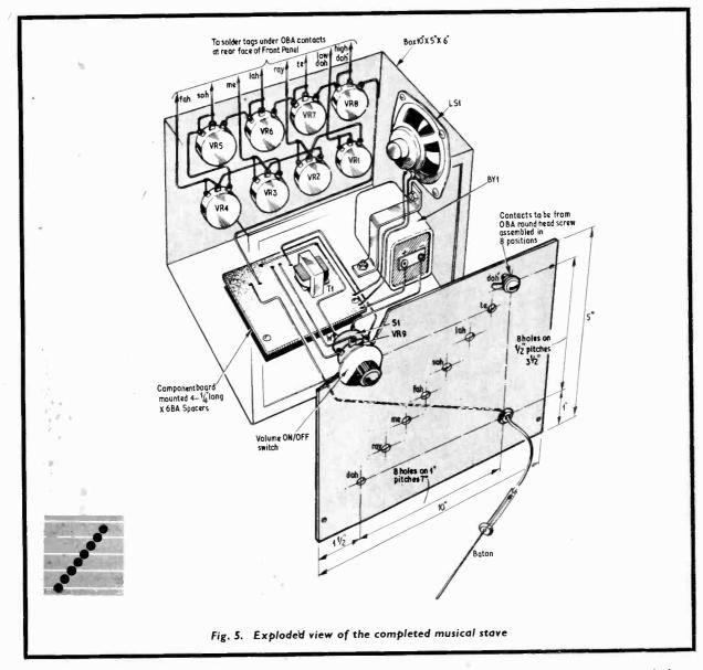
potentiometer VR1 is carefully adjusted to provide an identical note with the one on the piano.
