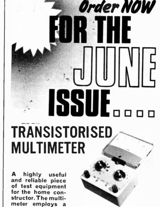
solid state amplifier to drive a moving coil meter, thus increasing the sensitivity of the meter by up to 100,000 times and at the same time protecting it against overload.
