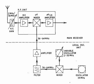
Fig. 8.1. Block schematic diagram of the local oscillator unit
