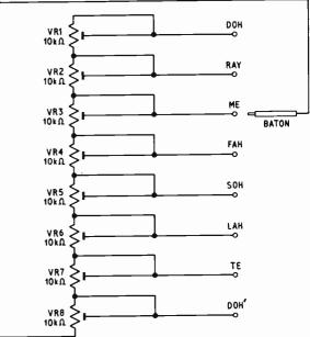
Fig. 2. Resistor chain used for varying frequency of tone generator
