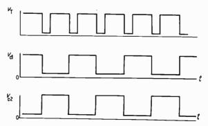
Fig. 6.3b. Waveforms for the binary divider
