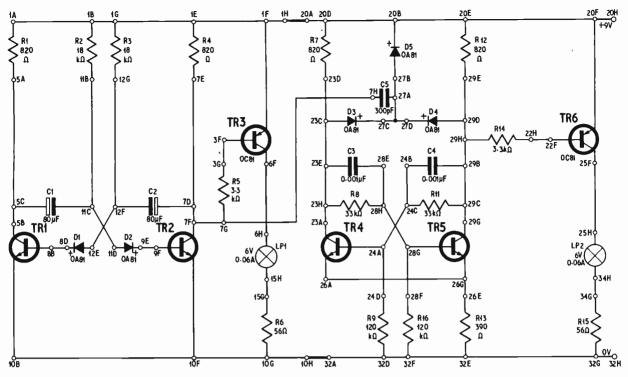
Fig. 6.4. Circuit of practical square wave generator and  $\div$ 2 divider with T-Dec connections
