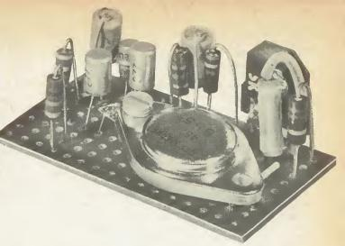
This unit gives a stabilised output voltage from an unstabilised input. The output can be varied between approximately 7 and 12 volts, at currents up to approximately 400mA, or up to 1A if the output transistor is mounted on a heat sink.
