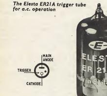
Fig. 3.1. Graphical symbol for a cold cathode trigger tube
