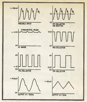
Fig. 4. Wave shapes at different stages of the circuit
