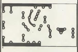
Fig. 2.9. Printed circuit board layout and wiring for oscillator assembly
