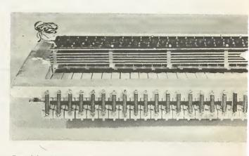
Fig. 2.2. Upper manual contact assembly shown in perspective with one hardwood strip removed
