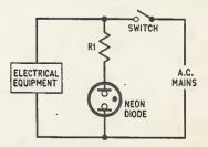
Fig. 2.1. Use of a symmetrical neon diode as a mains indicator
