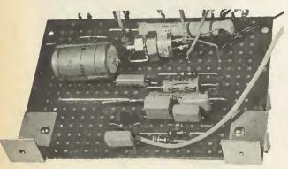
Photograph of board "A" showing the mounting brackets and position of components
