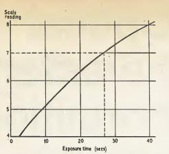
Fig. 5. Calibration graph for indicating exposure time against scale reading
