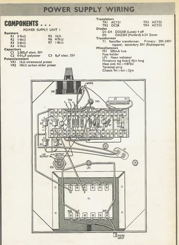
Fig. 2.5. Wiring layout for P.S.U.I. The d.c. output wires are taken to a terminal strip mounted on chassis top, see Fig. 2.6
