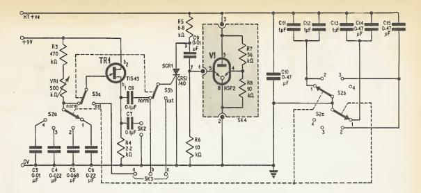
Fig. 1. Circuit diagram of the stroboscope not showing the power supply
