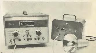
Set up for calibrating the stroboscope using a frequency meter-see text
