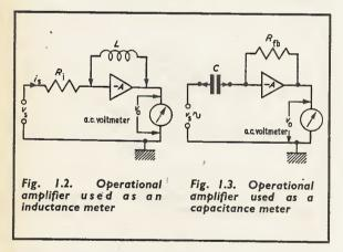
value, set the input alternating voltage at a suitable frequency and measure the output voltage on an r.m.s. reading a.c. voltmeter.
