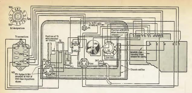
Fig. 6. Layout and wiring diagram of the complete stroboscope. Boards "A" and "B" and transformer TI are shown removed for clarity
