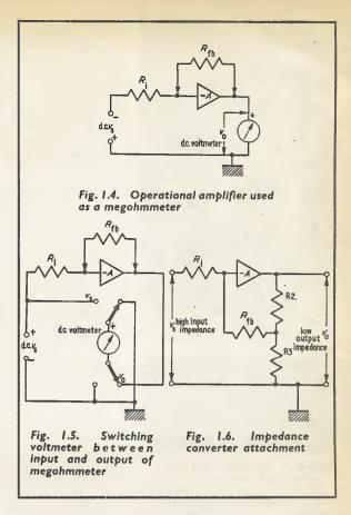
Notice that an accurate source of voltage is not required. Only the ratio  $v_0/v_s$  is required; this can be read by putting the meter across input and output terminals in turn (see Fig. 1.5).
