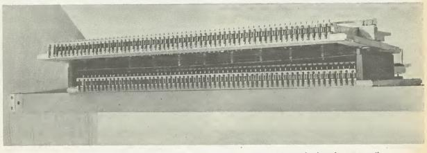
Fig. 2.3. Upper and lower manuals complete with contact units in position on keyboard support rails
