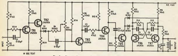
Fig. 3. Circuit diagram of the guitar bass-maker
