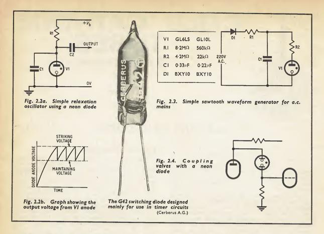
is negligible. After many thousands of hours of use the light emitted by a neon diode falls owing to sputtered material collecting on the envelope of the tube. The diode can then be replaced before total failure occurs.
