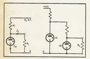
Fig. 2.5. Basic voltage stabiliser circuit Fig. 2.6. Cascaded stabiliser tubes
