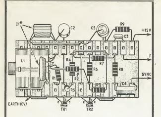
Fig. 2.8. Tagboard mounting and wiring of oscillator components
