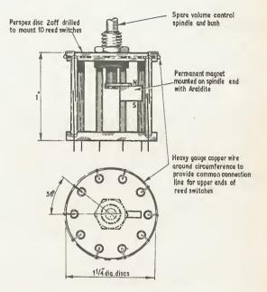
Fig. 2. Single-pole, 10-way reed switch
