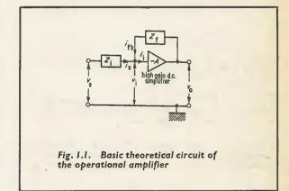
current  $i_i$  is very small indeed—in practice just a few millimicroamps. Consequently we can afford to ignore this in the calculation and put  $i_i$  as zero which simplifies the above equation to
