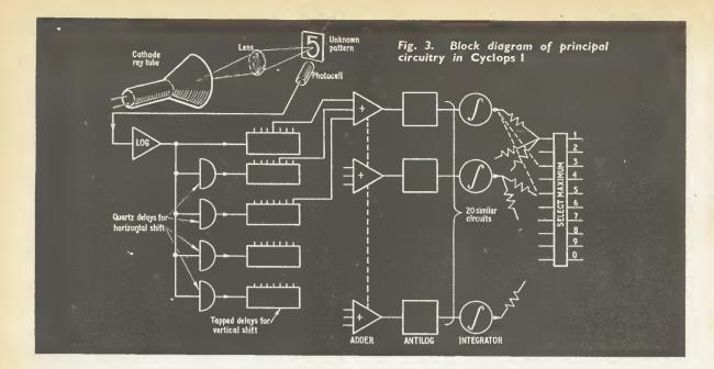
The process is analogous to that of training the resistive network, to which n-tuple measurements are applied, in the Cyclops system to modify itself when a wrong answer is obtained.
