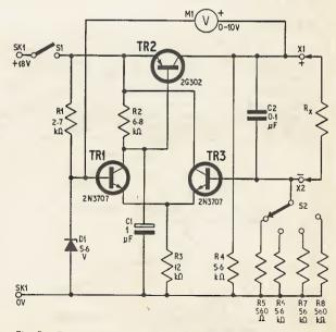
Fig. 5. Practical circuit of the linear scale ohmmeter
