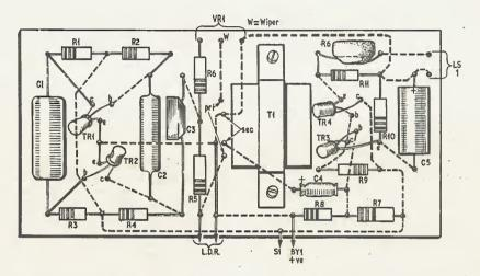
Fig. 2. Layout of components on the perforated wiring board. Underside wiring is shown as dotted lines
