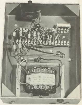
Chassis underside of power supply unit, see Fig. 2.5 for details
