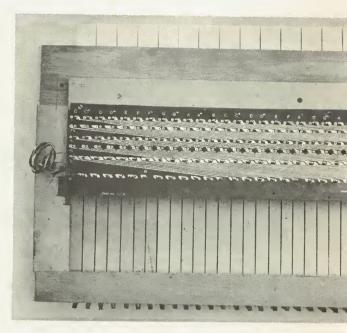
Fig. 2.1. View of the underside of the upper manual contact assembly showing the pitch connections to the printed circuit board. Note the hardwood strip which fixes the board to the keyframe
