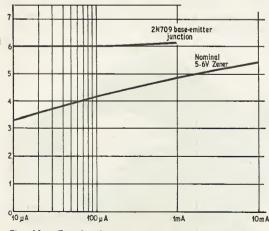
Fig. 10. Graph of results obtained when testing a 5.6V Zener diode and the base-emitter breakdown voltage of a 2N709 transistor
