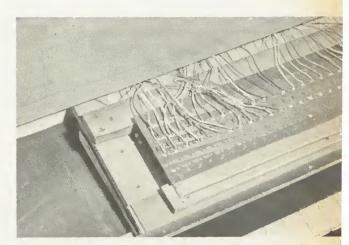
Underside of the lower manual showing printed board wired and mounted to keyframe via hardwood strips
