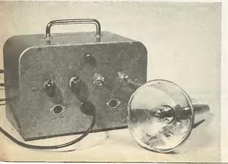
To supply the large amount of energy required for the flash, it is necessary to connect a capacitor (C10 to C15) across the tube between cathode and anode. Between flashes this capacitor charges up to supply potential, and during the flash it is rapidly discharged through the tube releasing all the stored energy in a very short period.
