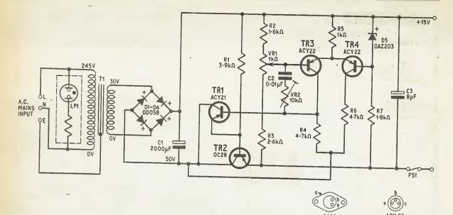
Fig. 2.4. Circuit diagram of power supply unit for generators and dividers
