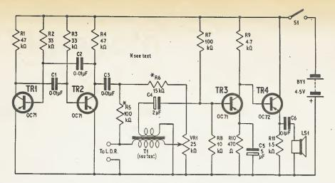
Fig. 1. Complete circuit of the enlarger exposure meter
