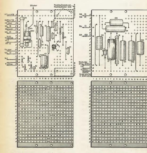
Fig. 4. Component layout and wiring of board "A"
