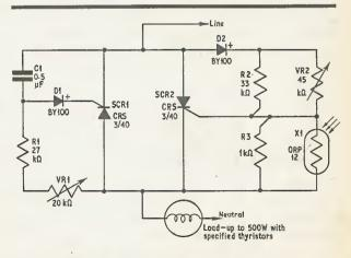
Fig. 1. Automatic spotlight control switch
