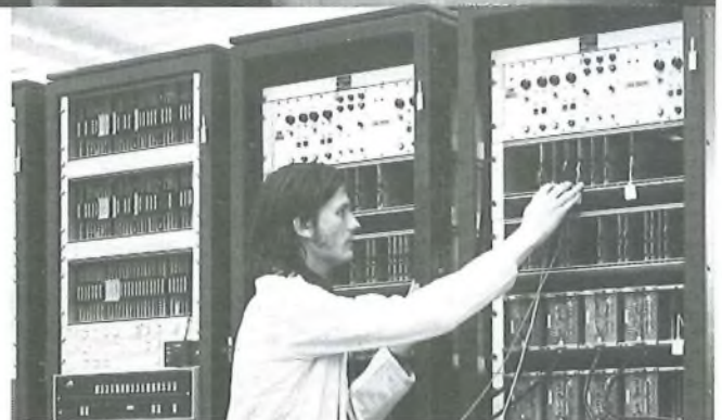
A Postcode translator undergoing final tests before delivery to the Post Office.
