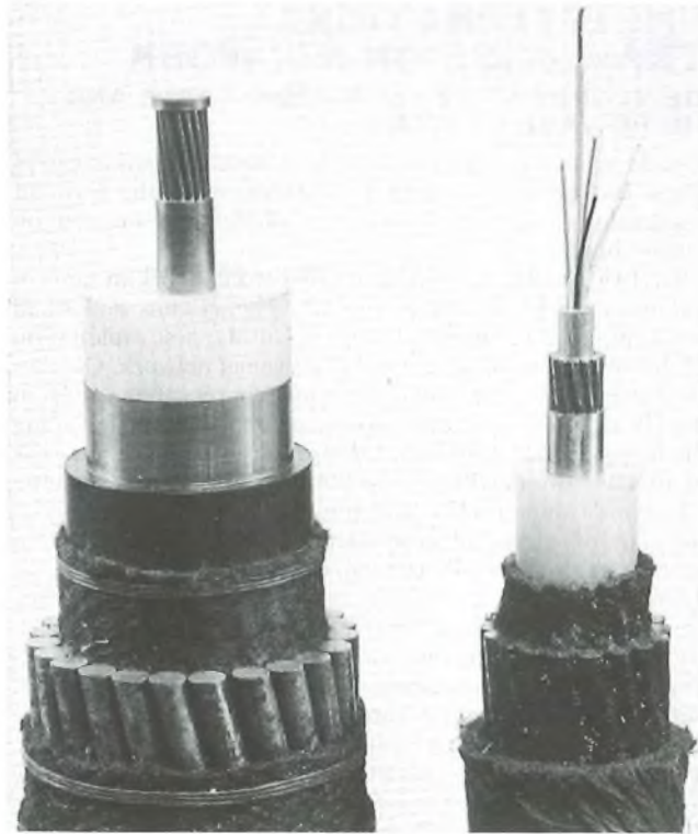
(a) SG -type coaxial cable (43 mm diameter) (b) Loch Fyne optical-fibre cable Note: The SG -type coaxial cable system has a capacity of 4000 circuits. Early optical-fibre cable systems have a capacity of 1920 circuits (140 Mbit/s) per fibre pair. The design shown allows a maximum of 5 pairs
