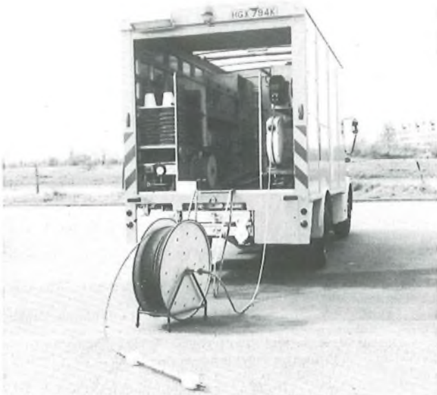
FIG. 17—Rodding and Light-Cabling Vehicle with duct motor in foreground
