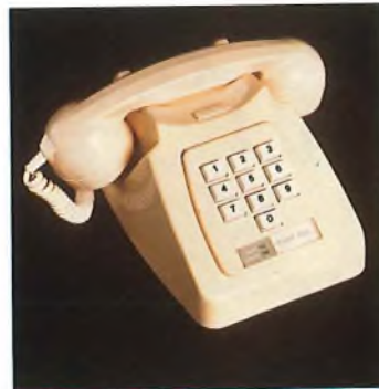
(h) Telephone No. 756 (self-contained press-button—3 × 3 + 1 configuration)—1975
