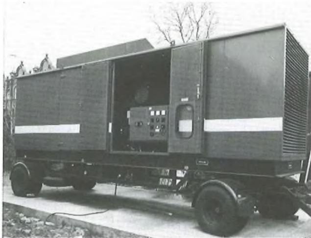
FIG. 5—Stand-by 250 kVA generator set mounted on a trailer
