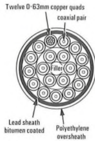
FIG. 7—Cable Coaxial, 18 pr/2.6/9.5 mm + 24 pr/0.63 mm
