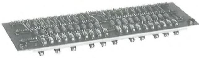
FIG. 4—Typical module of experimental PABX (1955) showing component mounting and interconnexion
