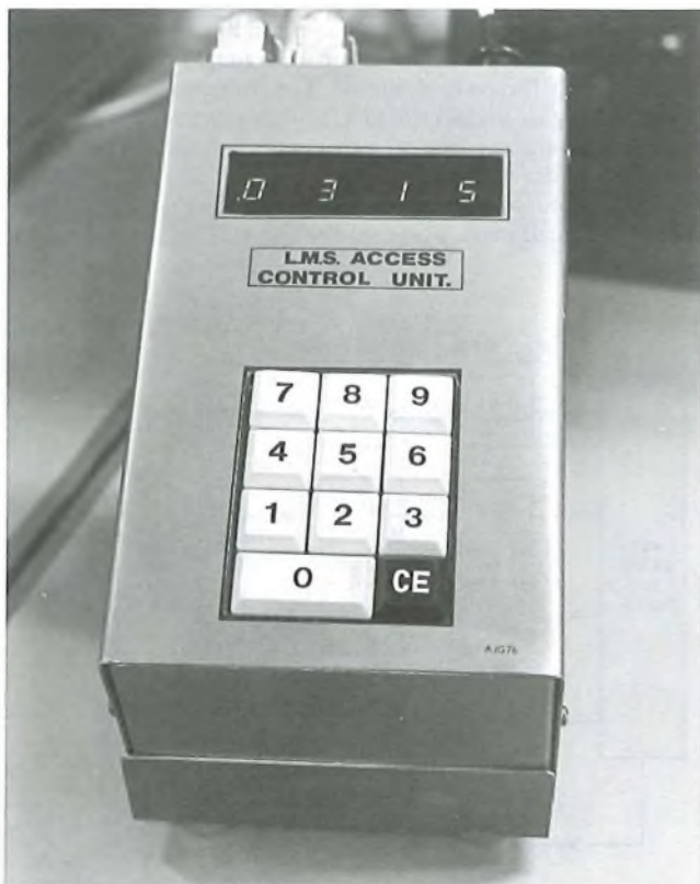
FIG. 4—Access control unit
