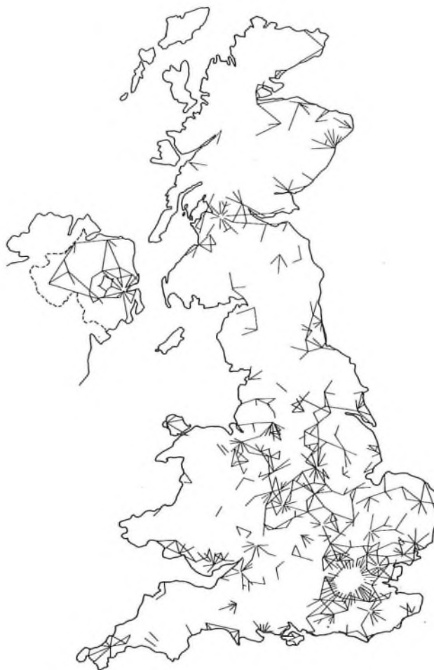
FIG. 1—British Post Office 24-channel PCM network at 1978 (7000 systems)
