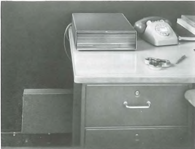
FIG. 2—Table-mounted modem unit with wall-mounted line unit
