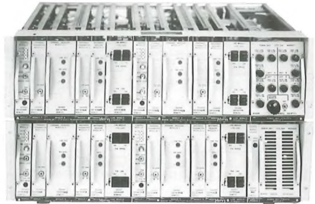
FIG. 3—Four modems and associated line equipment in rack-mounted form
