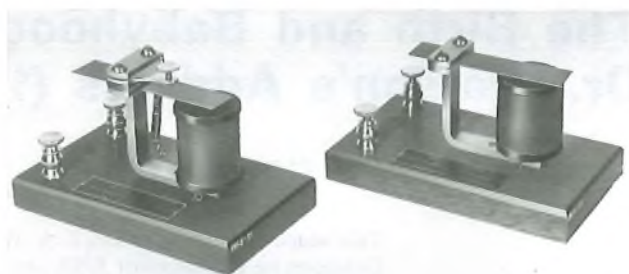
Replica of Bell's Harmonic Telegraph (Crown Copyright. Science Museum, London)
