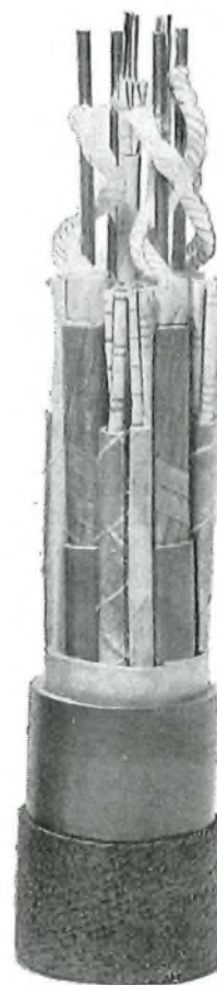
FIG. 1—The 1935 design of 3·0/11·4 mm (0·450 in) coaxial cable
