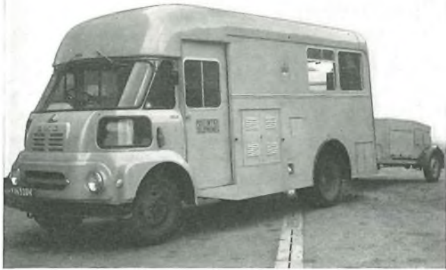
FIG. 5—New van complete with trailer generator
