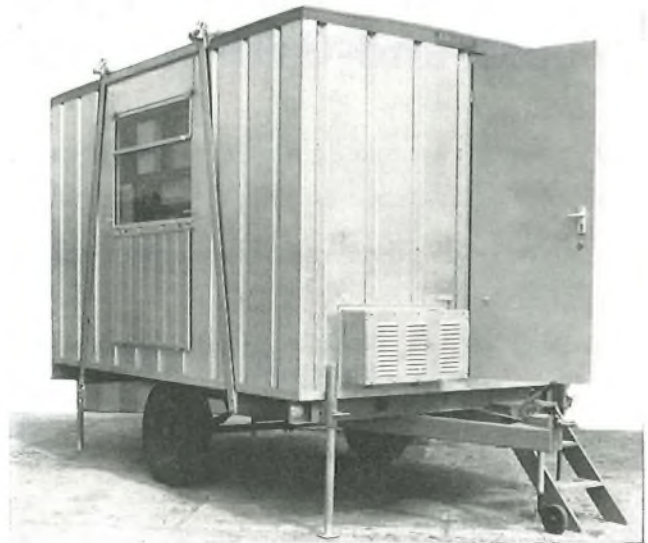
FIG. 6—External view of trailer caravan showing air conditioner intake
