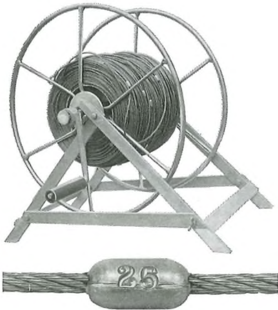
FIG. 8—Length-measuring device and close-up of ferrule
