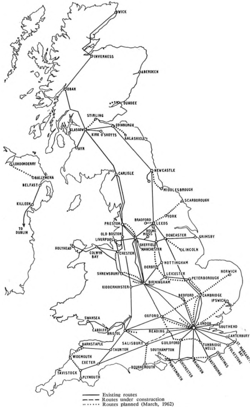
FIG. 3—UNITED KINGDOM COAXIAL-CABLE ROUTES, 1962
