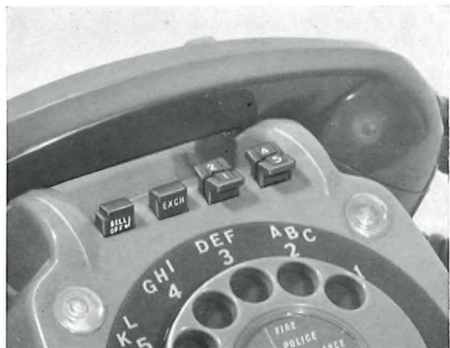
FIG. 3—PRESS-BUTTONS AND SUPERVISORY LAMPS ON INTERCOMMUNICATION TELEPHONE
