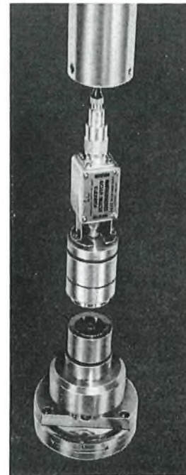
FIG. 2—LOWER AERIAL-MAST BEARING AND COAXIAL COUPLING
