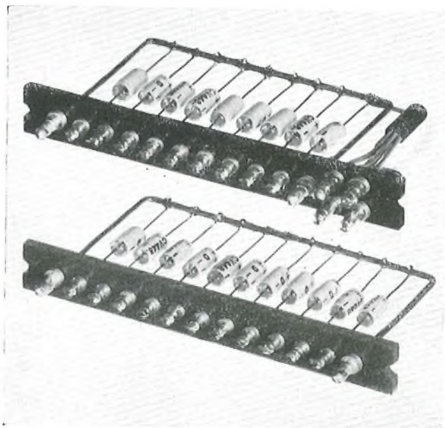
FIG. 10—FIRST "OR" GATE AND AMPLIFIER
