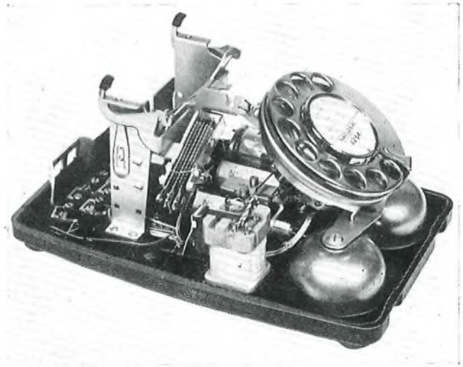
FIG. 8—INTERIOR OF CONVENTIONALLY-WIRED TELEPHONE
