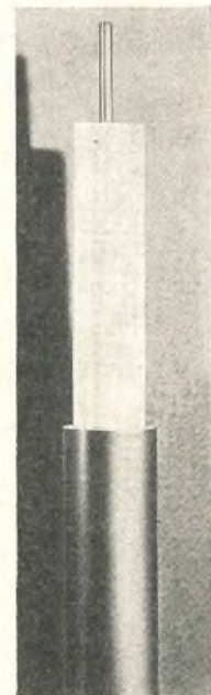
FIG. 1—TYPICAL SOLID-POLYTHENE-INSULATED LEAD-SHEATHED RADIO-FREQUENCY CABLE. APPROXIMATE OVERALL DIAMETER 1 IN. ATTENUATION 0.9 DB/100 FT AT 100 MC/S
