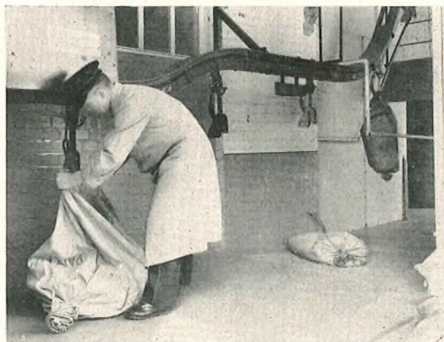
FIG. 6—CHAIN-CONVEYOR LOADING POINT AT LEAMINGTON SPA SORTING OFFICE
