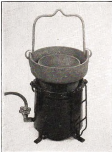
FIG. 3.—GAS FURNACE AND PLUMBER'S POT.
