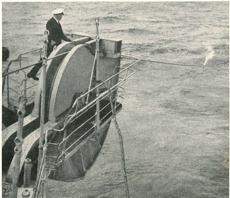
FIG. 9.—CABLE PAY-OUT OVER THE STERN SHEAVE.
