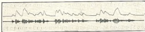
FIG. 1.—WAVEFORM OF SPEECH (LOWER TRACE) AND CORRESPONDING DEFLECTIONS OF VOLTMETER NEEDLE (UPPER TRACE).
