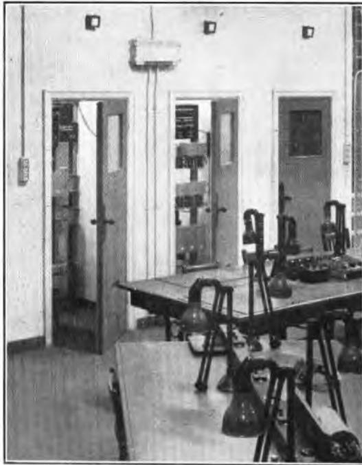
FIG. 3.—CUBICLES FOR MECHANICAL PERFORMANCE LIFE TESTS.
