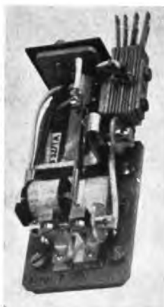
TYPE 89 HIGH-SPEED RELAY with single changeover.
