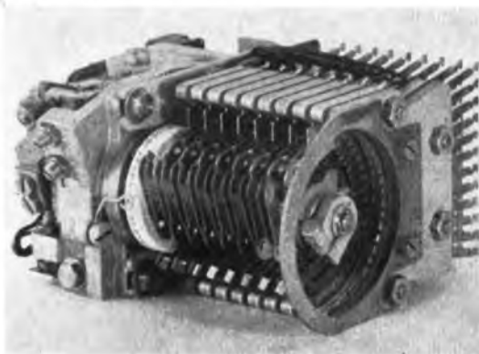
MOTOR UNISELECTOR operates at 200 steps per second.
