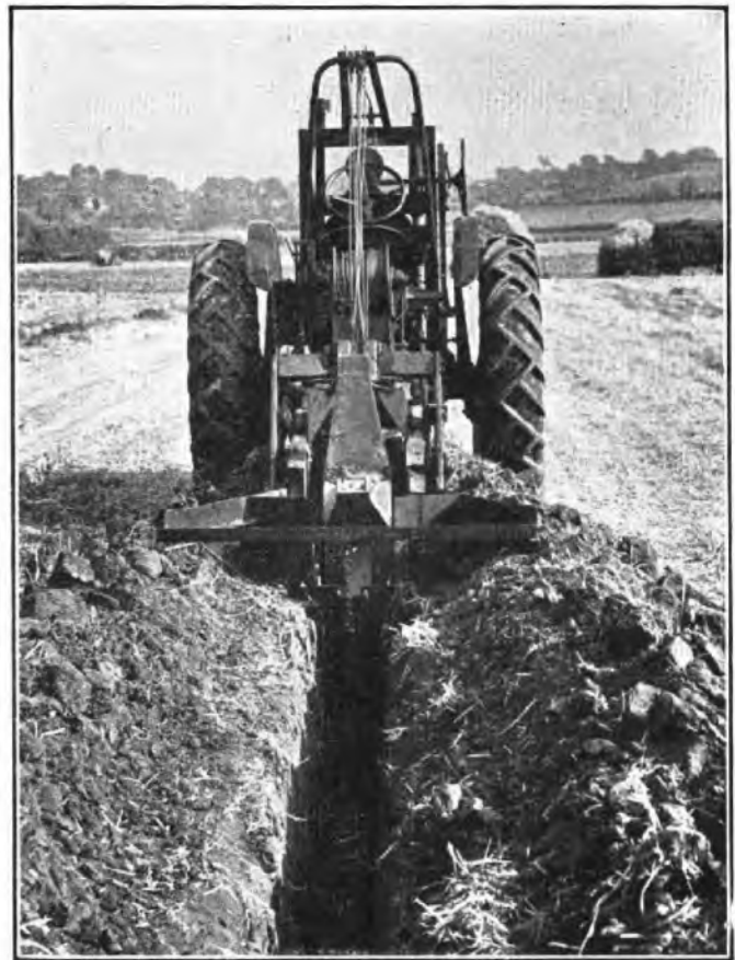
REAR VIEW OF AVELING BARFORD TRENCHING MACHINE TYPE HA2.
