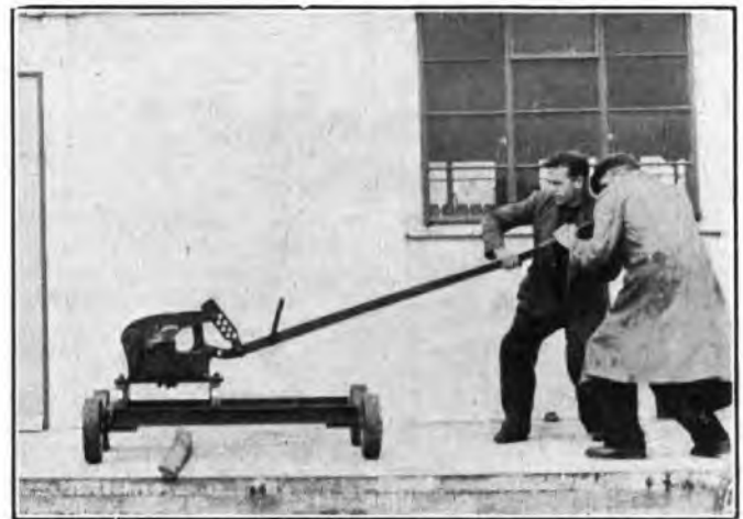
CUTTING CABLE WITH THE GUILLOTINE.
