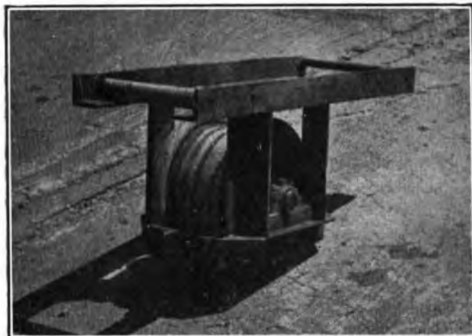
THE "MORRIS WHEEL," CONSTRUCTED USING A 15-IN. X 9-IN. ARMY TRUCK WHEEL.
