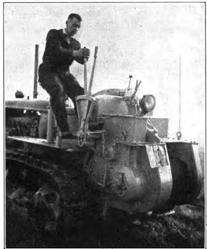
REAR VIEW OF TRACTOR WINCH, SHOWING CONTROL LEVERS AFTER MODIFICATION.
