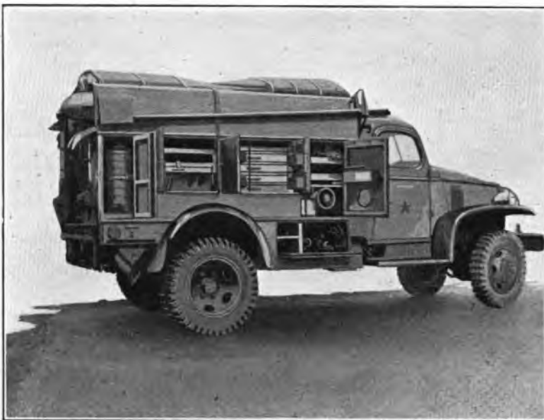
FIG. 3.—LINE CONSTRUCTION TRUCK.
