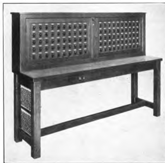
FIG. 7.—MASTER CONTROL PANEL FOR DISTRIBUTION OF ANNOUNCEMENTS.
