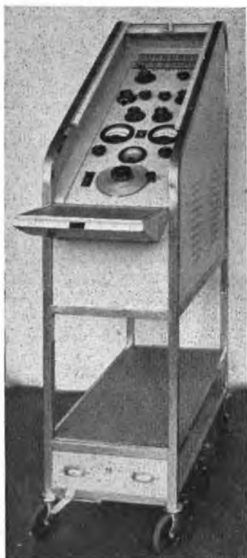
FIG. 6.—TROLLEY-MOUNTED TEST UNIT.
