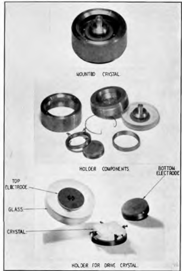
FIG. 25.—DRIVE CRYSTAL AND COMPONENTS.
