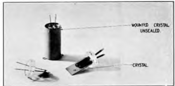
FIG. 16.—HOLDER FOR CHANNEL FILTER CRYSTAL RESONATOR
