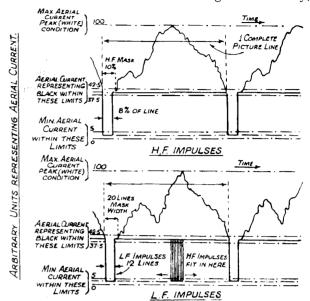
Fig. 3.—Waveform of Transmitted Signal, Sequential Scanning System.
