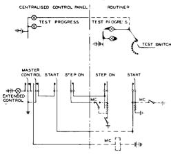
Fig. 2.—Circuit showing Principle of Centralised Control and Display.
