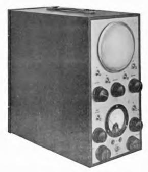
THE "Standard" 74320 Cathode Ray Oscillograph is a portable, self-contained equipment operating from A.C. mains, and incorporating a linear time base suitable for viewing waves from 15 to 500,000 p.s. It includes a single stage amplifier, accurately linear for outputs covering the whole screen, the gain of which is 17 db.  $\pm \frac{1}{2}$  db. (7:1) from 15 to 15,000 p.s.
