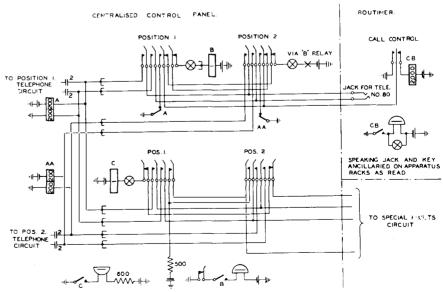
Fig. 3.—Typical Speaking and Signalling Circuits between Control Positions AND (A) ROUTINERS, (B) FAULT REPORTING CIRCUITS.
