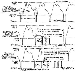
Fig. 5.—Waveform of Transmitted Signal, Interlaced Scanning System.
