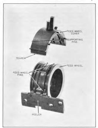
Fig. 6. FEED WHEEL AND ASSOCIATED PARTS.
