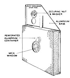
FIG. 11.—SILCA GEL DEHYDRATOR.
