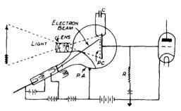
Fig. 15a.—Principle of the Iconoscope.
