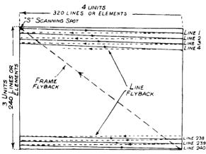
FIG. 2.—SEQUENTIAL SCANNING.
