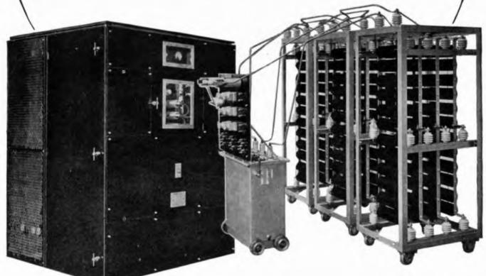
Above is illustrated an H.T. supply unit with an output of 6,000 volts I A, smoothed 0.03 per cent, ripple, supplied to the New Zealand Government. This type is specially finished to match the radio equipment, and includes rectifier, mains transformer and full protective and alarm circuits. On the right is a 5.000 V 2 A unit of the simplified construction type and includes rectifier and mains transformer only.
