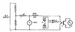
Fig. 8. -Circuit of LMW Calibration Unit.
