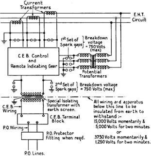
Fig. 18.—Schematic Diagram of Connections of P.O.
