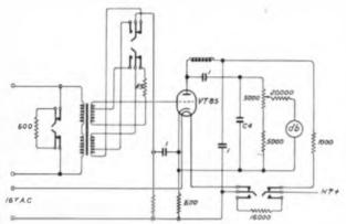
Fig. 5.—Simplified Circuit of Transmission Measuring Set.
