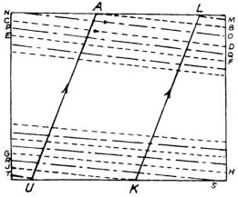
Fig. 4.—Interlaced Scanning.
