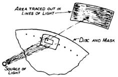
Fig. 6.—Spotlight Method of Scanning.
