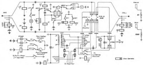
Fig. 7.—Phonogram Operator's Cord and Telephone Circuit.
