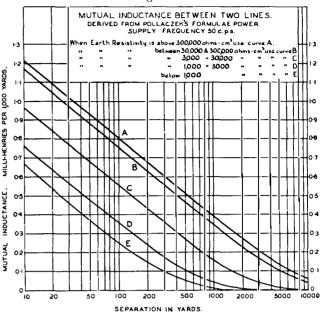
Fig. 3.—Curves for the Calculation of Mutual Inductance.
