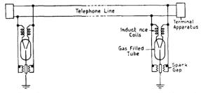
Fig. **6a.**—Diagrammatic Arrangement of Two Gas-Filled Discharge Tubes connected to a Telephone Line.
