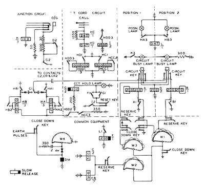
Fig. 5.—Distribution Position Circuit.
