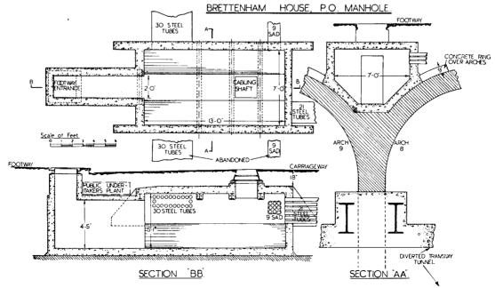
Fig. 3.—Details of specially designed Reinforced Concrete Manhole.
