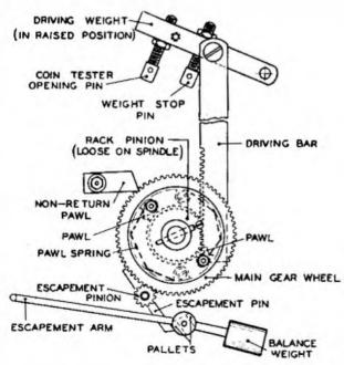
Fig. 2.—Drive and Escapement Mechanism, Type B4
