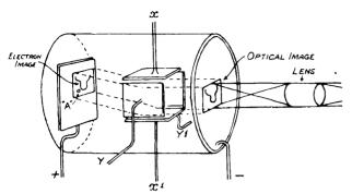
FIG. 10.—PRINCIPLE OF THE ELECTRON CAMERA.
