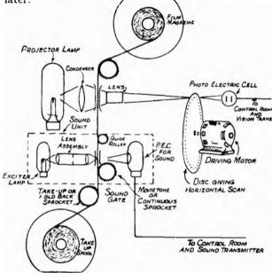
FIG. 7.—FILM SCANNING BY THE SPOTLIGHT METHOD.
