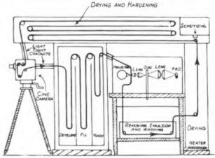
Fig. 9.—Schematic View of an Intermediate Film Transmitter.
