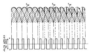
FIG. 13.—MERCURY ARC RECTIFIER. EFFECT UPON THE AMPLITUDE OF THE RIPPLE OF VOLTAGE REGULATION BY GRID CONTROL. EM GIVES THE AVERAGE D.C. VOLTAGES CORRESPONDING TO DIFFERENT DEGREES OF GRID CONTROL.
