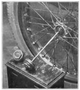
FIG. 2. - METHOD OF DRIVE FROM SIDECAR WHEEL.
