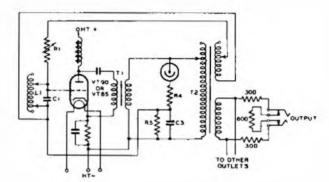
Fig. 1.—Simplified Circuit of Constant Output Oscillator.
