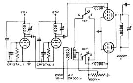
FIG. 1.—SCHEMATIC DIPLEX TRANSMITTING CIRCUIT.
