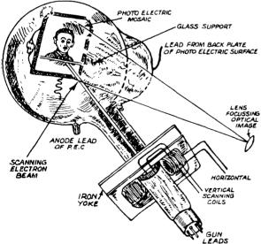
Fig. 14.—The Iconoscope.
