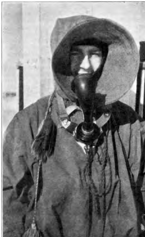
PART OF THE TELEPHONE EQUIPMENT USED IN THE AURORAL PHOTOGRAPHIC WORK. THE HEADGEAR RECEIVER IS WORN UNDER THE BURBERRY WINDPROOF HELMET AND OVER THE WOOLLEN BALACLAVA.
