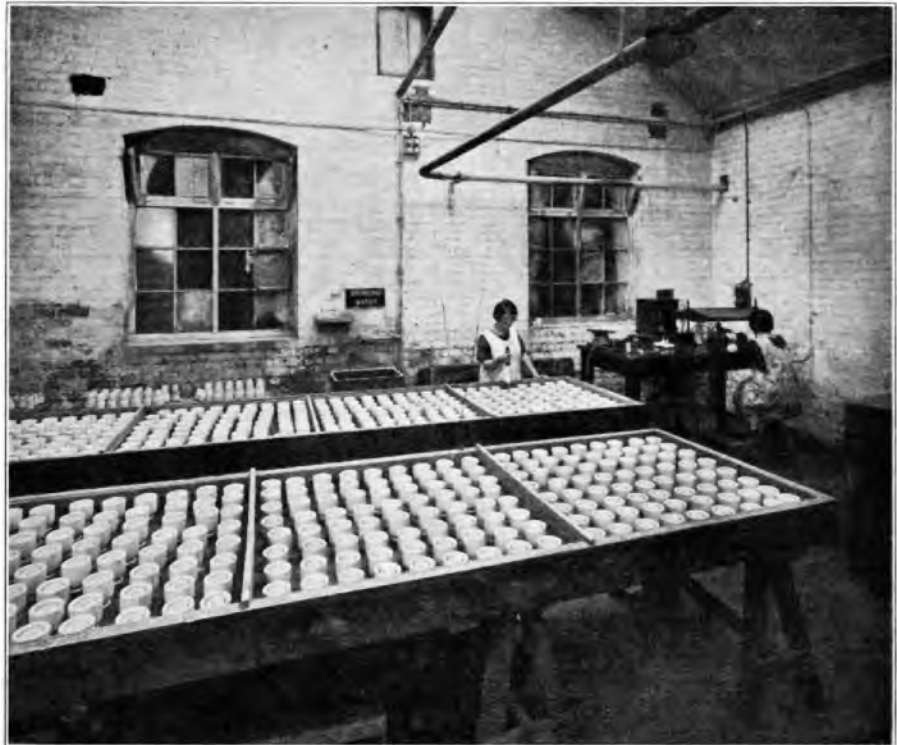
FIG. 5.—ELECTRICAL TESTING OF INSULATORS.
