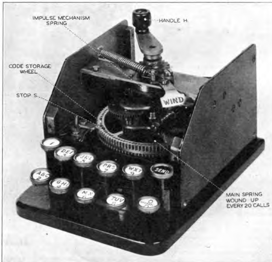
FIG. 14.—FIRST MODEL KEYSENDER.
