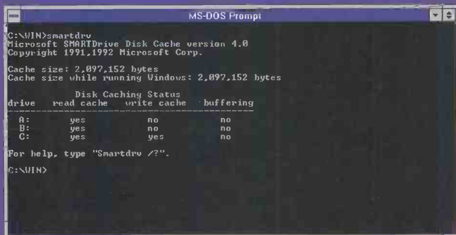
MS-DOS has a built-in cache called Smart Drive which will increase data throughput.
