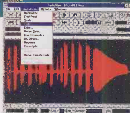
Voyetra's Audio View software includes a wave editor, audio mixer and CD-ROM controller and works with a wide range of PC sound cards.
