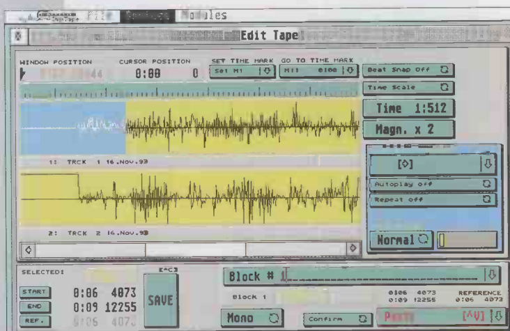
The Edit window lets you zoom in and edit up to two tracks at a time. You can link tracks to preserve stereo pairs.
