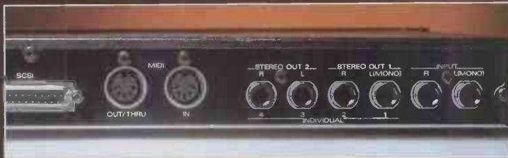
A slimmed-down rear panel with less outputs but a SCSI port for extra flexibility, and room for upgrades
