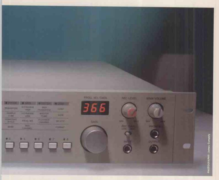
movements), and a Data Entry knob is used to actually change the parameter values. The S01 bears some relation to the \$700 in its use of sample 'banks'; however, where the S700 had six banks, the S01 has eight.
