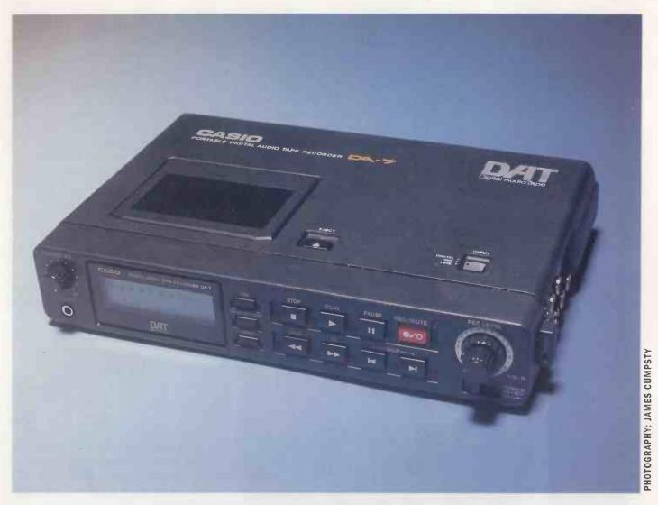
(more about this later). Once this is complete, the unit is ready to record - press Play to begin recording. While in Record Pause mode (after the recording of sub-code data), the record levels may be set using the ganged pots on the front panel - remember that even slighty overloading a digital recording produces unpleasant distortion rather than the tape compression characteristic of analogue systems.
