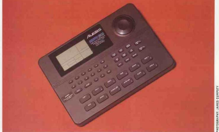
The compact dimensions of Alesis' latest drum machine belie the power lurking within - 233 16-bit drum and percussion sounds and innovative programming features make the SR16 a serious beatbox. Review by Simon Trask.
