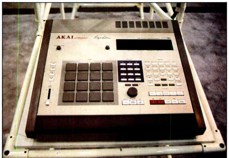
First machine to result from the collaboration between Akai and Roger Linn is the ADR15, a sampling percussion system in the Linn 9000 mould. A MIDI sequencer, the ASQ10, is to follow.
