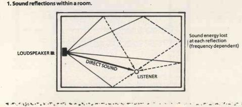
tend to die away fairly rapidly as the sound energy is converted into heat. And seeing as high frequencies tend to be absorbed more readily than low ones, the highfrequency part of the sound decays more rapidly than the low frequency part. Then there's the fact that because the air itself absorbs high frequencies due to the viscosity of the molecules, it's clear that the further the sound travels, the lower its high frequency content will be.
