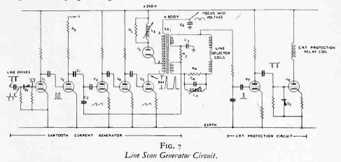
To maintain the same sawtooth amplitude at  $V_3$  when changing the TV system from either 405 to 625 or 525 lines, it is necessary to reduce the charging resistance by shorting out  $R_2$ .
