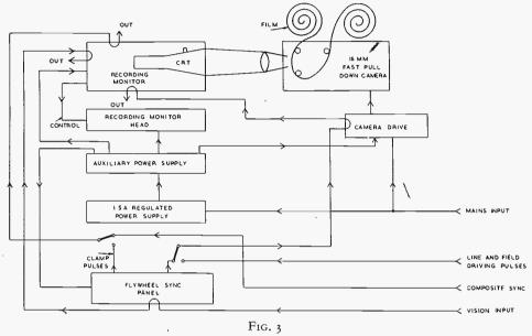
Block Diagram of Recording Channel.
