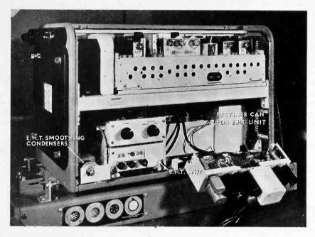
FIG. 4 Recording Monitor.
