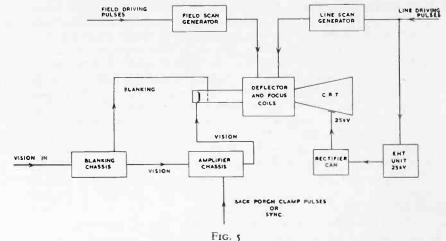
Block diagram of Recording Monitor.
