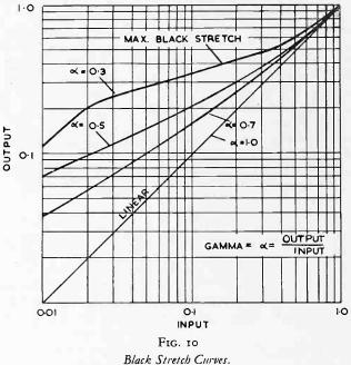
is not conducting and during the white parts it is conducting. The gain in the blacks is controlled by the variable resistance  $R_1$  which is connected across the diode  $D_1$ . The range over which the black stretch becomes effective is controlled by  $R_2$  which alters the bias of  $V_{15}$ .
