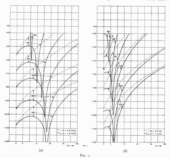
Maximally flat triple tuned circuit. Second barmonic distortion for negative detuning (a)  $\delta = \pm 0.002$ ; (b)  $\delta = \pm 0.01$
