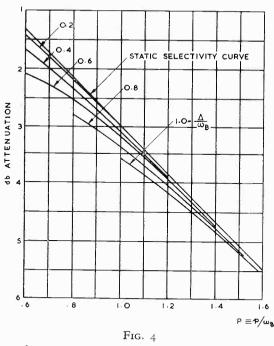
Output signal attenuation for the single tuned circuit
