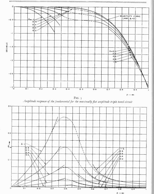
FIG. 6 Relative phase response of the fundamental for the maximally flat amplitude triple tuned circuit (132)
