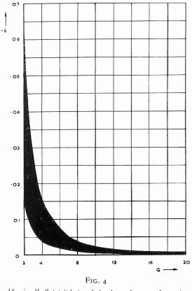
Maximally flat triple tuned circuit. Amount of negative detuning for minimum second harmonic distortion
