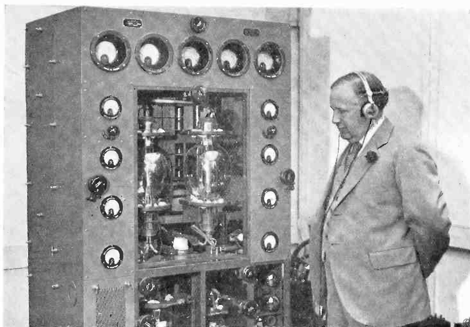
Sir Kingsley Wood, the British Postmaster-General, inspecting a Marconi short-wave telephone transmitter—of the type installed on passenger liners for ship-to-shore telephone services—at the recent National Radio Exhibition at Olympia, London.
