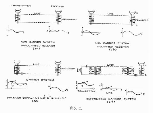
Fig. 1b shows a receiver with improved mentality, by polarisation with permanent flux, and in this case the reversal of current is now observed and correct reproduction results.
