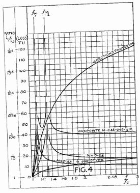
In passing, it should be noted that  $f_c$ , the frequency of cut-off does not mean that at the frequency  $f_c$  attenuation is present. In an ideal filter  $f_c$  is the boundary at which the pass region ends and the attenuation begins; hence the attenuation starts from zero at the frequency of cut-off.
