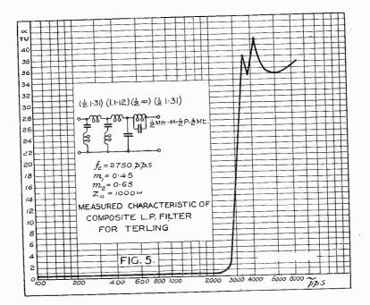
The derivation of such a type of section is rendered easy by the use of a parameter "m," which is determined from a knowledge of the frequency of cut-off and the frequency at which infinite attenuation is required. The properties of the
