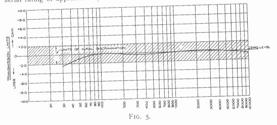
A frequency characteristic of this set is given in Fig. 5. It will be observed that this curve from 40 to 10,000 cycles is within 2 T.U. of the zero line, or alternatively, does not vary more than plus or minus 1 T.U. about a mean value. This degree of linearity means that over the frequency band mentioned the ear will be unable to detect any difference in amplitude, and consequently the curve can be considered flat over this range.
