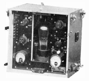
A.D.21 Transmitter. Front View. Variable air dielectric condenser operated from the front of the set. A tapping on the closed circuit inductance is connected to earth.
