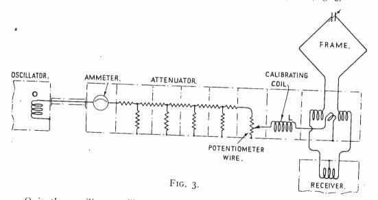
O is the auxiliary oscillator capable of supplying current at any desired frequency in the wave band (14 - 5,000).
