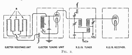
The ejector tuning unit will be seen to utilise an S.625 Valve. For duplex working the aerial is connected to the grid circuit (LC) of the tuning unit via the resistance unit R. The tuning range of this grid circuit is 300-4,000 metres, which covers the waveranges of all the types of transmitters with which it is intended for use. The anode circuit of the ejector valve is what corresponds to the aerial circuit of the R.G.19 in simplex working. It is therefore tunable over the receiver waverange.
