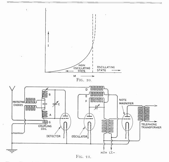
The oscillator is simply a tuned anode oscillator tuned to about 20,000  $\sim$  per second. A coupling coil D is in series with the H.T. supply to the detector. When the oscillator impresses a varying E.M.F. on this coil, the H.T. voltage on the detector is varied at a super-sonic rate, and causes this valve to start and stop oscillating, at a frequency of 20,000  $\sim$  per second.
