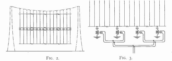
The limitation imposed on the concentration of the beam by the economic restriction on the size of parabolic reflectors was removed by adopting this type of construction, the ground area covered by the masts, reflector and aerial for a system of 2 wavelengths' aperture being now only  $\frac{1}{10}$  what was formerly required.
