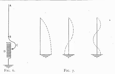
Now since the current in such an aerial is due to the passage of electrons into and out of a capacity, and since this capacity must be zero at A, and maximum at the earth end of the inductance; it follows that the current must be zero at A, and maximum at earth. Therefore if we wish the aerial to resonate (i.e. to radiate maximum energy) at a wavelength  $\lambda$ , it is obvious that the effective length of the aerial and loading inductance must be
