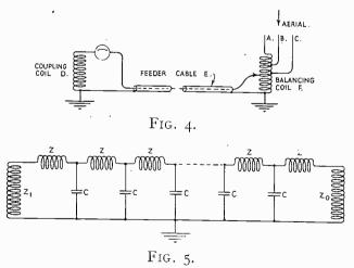
Now such a lead covered cable, terminated at its two ends by impedances
