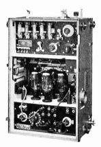
Marconi A.D.6h Aircraft Wireless Set. built for the British Air Ministry by Marconi's Wireless Telegraph Company, and in its construction were combined the results of the experience and technical knowledge of the British Air Ministry, and of the Marconi Company.
