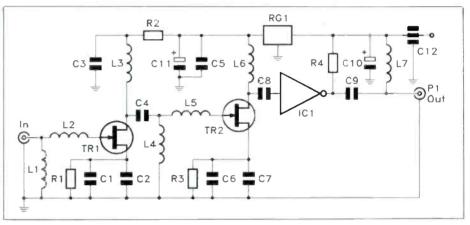
Figure 4. Pre-amplifier circuit.
