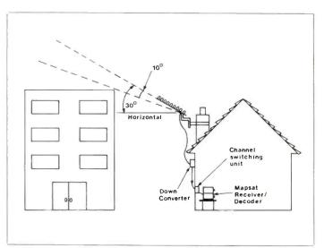
Figure 6. Aerial azimuth.
