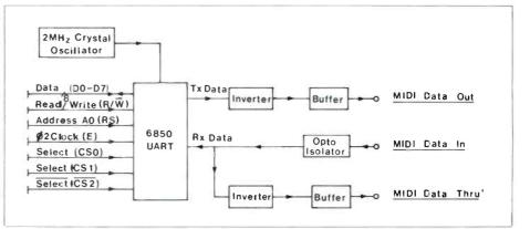
Figure 1. Block diagram.
