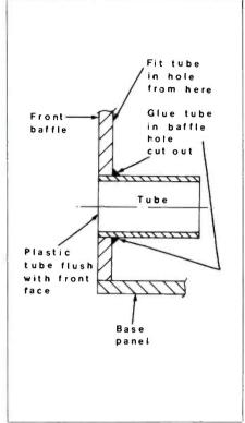
Figure 11. Fitting the port tube.
