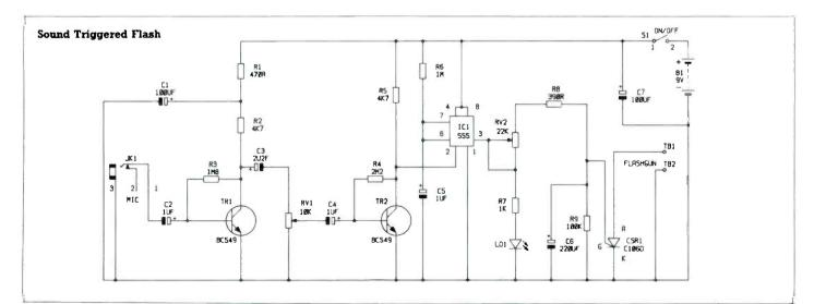
kind. In this case a two stage common emitter amplifier is used, and this provides over 80dB of voltage gain. RV1 is the gain control, and it is generally advisable to have the gain no higher than is really necessary as this would almost certainly result in frequent spurious triggering of flashgun, and possibly a lot of wasted frames.
