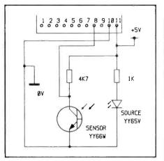
Figure 4. Opto-coupled input.
