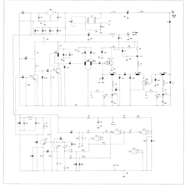
Figure 5. Down Converter circuit.
