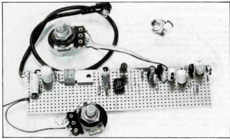
microphone (the type used with inexpensive cassette recorders), although it will function reasonably well with crystal, high impedance dynamic types, or types which have similar output characteristics to the latter. With any of these types of microphone the output level is only going to be something in the region of 1 millivolt, and a considerable amount of amplification is needed in order to boost the signal to a level that can drive a switching device of some
