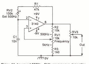
Figure 11. Improved 500Hz - 5kHz squarewave generator.
