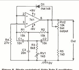
Figure 8. Diode-regulated 1kHz Twin-T oscillator.
