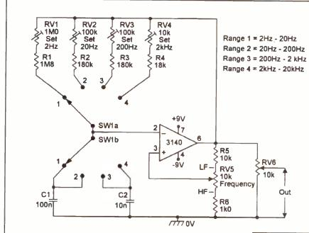
Figure 12. 4-decade, 2Hz - 20kHz, squarewave generator.
