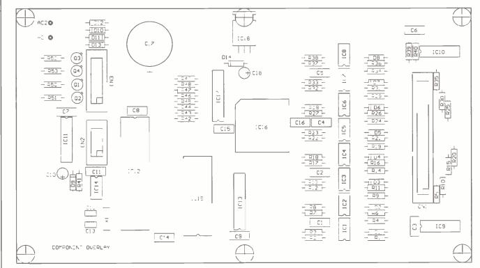
Figure 16. Component overlay for the main PCB. Take particular note of the orientation of the ICs, diodes and electrolytic capacitors. Note: Figure shown at 85%
