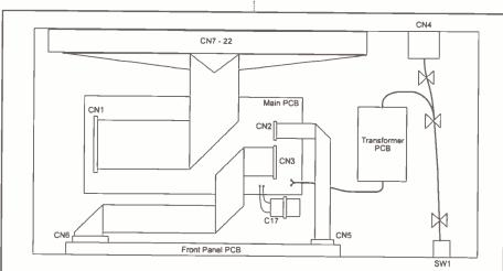
Figure 20 Internal layout. Careful folding of the ribbon cables ensures a neat layout. The mains wiring should be secured to the case at the points shown. C17 is secured with a cable tie and clip next to the main PCB.
