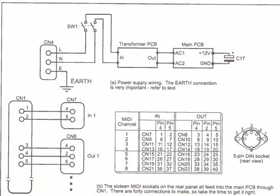
Figure 21 Internal wiring diagram showing (a) power supply wiring and (b) MIDI signal wiring from CN1 to the rear MIDI sockets.
