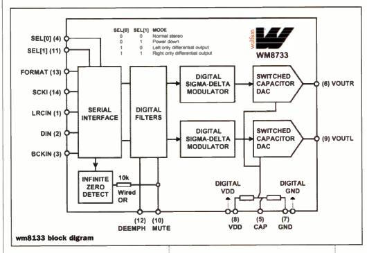
problem. The MN66710's audio decoder is coupled to a Wolfson WM8733. This sigmadelta stereo DAC is capable of working at 24bit/96kHz, and is thus possibly over-specified as far as DAB is concerned. There are two WM8733s, the second one being concerned with providing fine-tuning voltages to the front end. Controlling the whole show is a 16bit microprocessor, which is also sourced from Panasonic. A rechargeable battery
