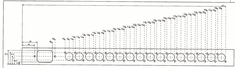
Figure 19 Rear panel mechanical drilling details. All small holes are 3mm in diameter; the larger round holes are 15.5mm in diameter. The cut-out for the IEC mains connector has 5mm radiused corners.
