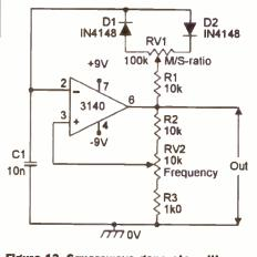
Figure 13. Squarewave generator with variable M/S-ratio and frequency.
