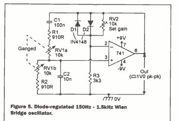
and reduces its resistance, thereby automatically reducing the circuit's gain and stabilizing the amplitude of the output signal.
