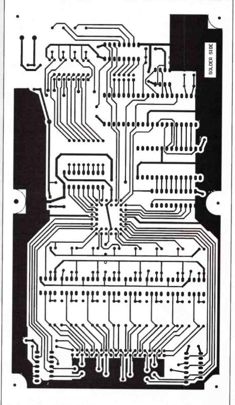
Figure 22a. Solderside foil pattern
