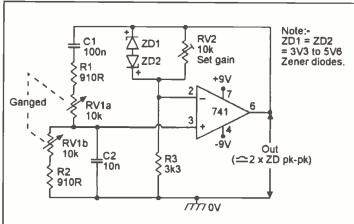
Figure 6. Zener-regulated 150Hz - 1.5kHz Wien Bridge oscillator.
