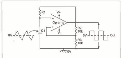
Figure 9. Basic relaxation oscillator circuit.
