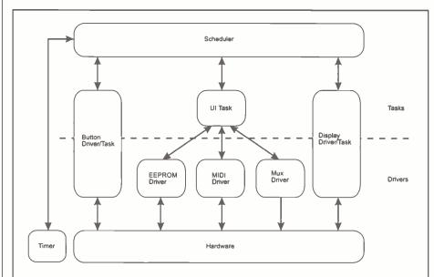
Figure 10. The modular software approach simplifies design, debugging and testing
