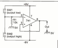
Figure 18. Simple manually-triggered bistable.
