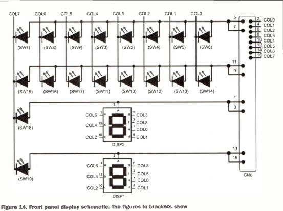
which buttons the LEDs are mounted in.
