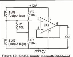
Figure 19. Single-supply manually-triggered bistable.
