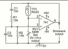
Figure 3. Thermistor stabilized 1kHz Wien Bridge oscillator.
